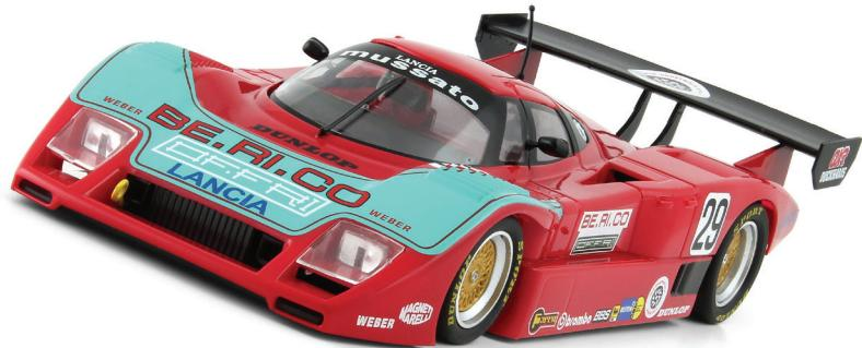
Hewland gearbox, 5 gears. The wheels diameter was 15 inches at the front and 17 at the rear. Chassis was made of aluminum and magnesium; body material was carbon fibre composite. The overall weight was 850 kg. Often, Lancias were as competitive as Porsches, in pure speed, but then suffered troubles at longer distances.
